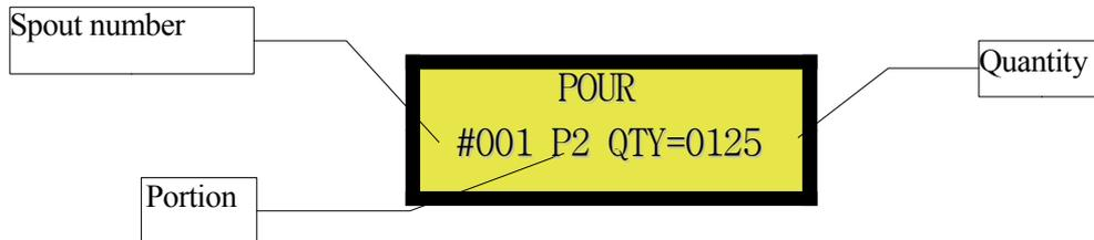
The quantity is hundredths of an ounce or milliliters, depending on the option selected. The unit will stop pouring when the specified quantity is reached. However, if you stop pouring before the set quantity has been reached, a full portion will still be registered.
