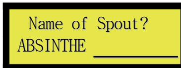
Using keys P1 to P4, text can be edited from left to right, moving through the word. Press P1 to change the font.
