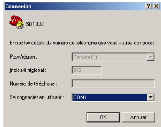
Give your connection a name, and press OK. Then select the communication port. The communication port must be the port you are using to communicate.
